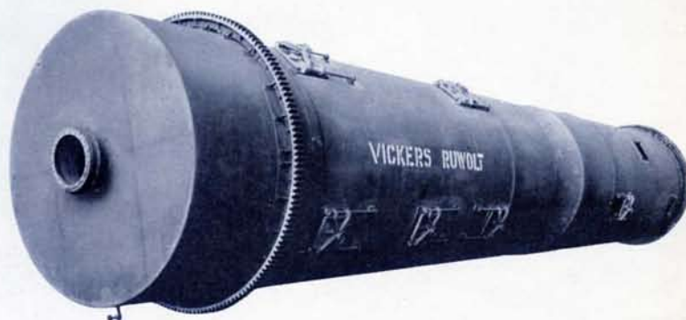
Portion of a 12-drum Malt Germinating plant, supplied complete with air-conditioning and kilning equipment.
